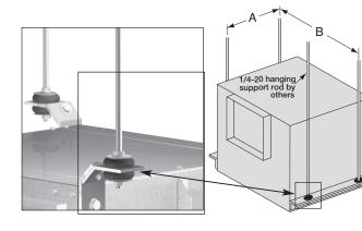
Vibration isolator kits are available for suspended installations. Kits include all hardware necessary to mount one unit, with the exception of <sup>1</sup>/4-20 threaded rod to be supplied by others. Fan mounting brackets include prepunched mounting holes for ease of installation.
