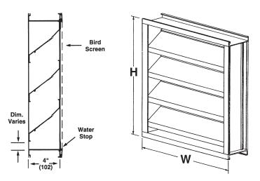
FRAME CONSTRUCTION Box frame or Flanged (Front or Rear)
