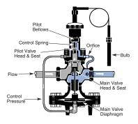
The Spirax Sarco pilot operated temperature regulator works by converting the process temperature to a force which is balanced by the control spring. This modulates a small valve head over a seat (the pilot). The flow through this seat is directed in turn to the main valve diaphragm, where it modulates the main valve.
