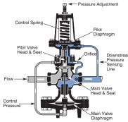
The Spriax Sarco pilot operated pressure regulator works by balancing the downstream pressure against a control spring. This modulates a small valve head over a seat (the pilot). The flow through this seat is directed, in turn, to the main valve diaphragm, where it modulates the main valve.
